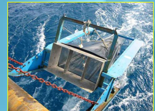
Fig. 2 - The suprabenthic sledge used for the experimental hauls.
